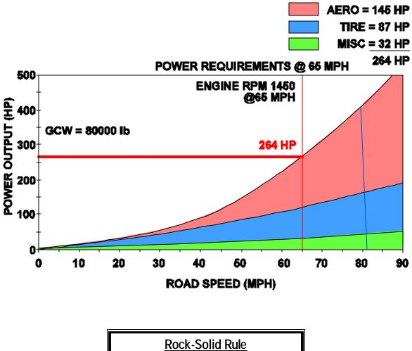
Tires make biggest difference in mpg below around 50 mph; aerodynamics is the most important factor over 50 mph.
